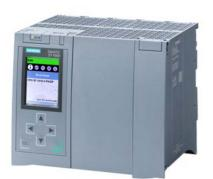
\*\*\* spare part \*\*\* SIMATIC S7-1500, CPU 1518-4 PN/DP ODK, central processing unit with ODK runtime interface, work memory 6 MB for program and 60 MB for data, 1st interface: PROFINET IRT with 2-port switch, 2nd interface: PROFINET RT, 3rd interface: PROFINET basic services, 4th interface: PROFIBUS, 1 ns bit performance, SIMATIC Memory Card required
